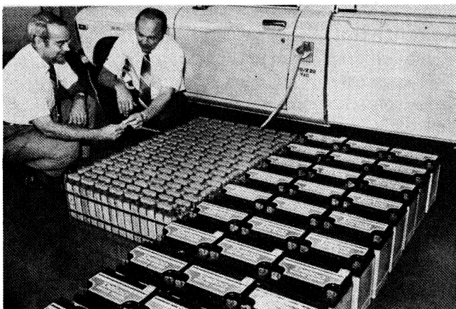
ELECTRIC BATTERY PROGRESS. This size comparison illustrates progress made on GM's new zinc-nickel oxide batteries, located at the left. The new battery pack is only half as large, and at 900 pounds, weighs less than half as
