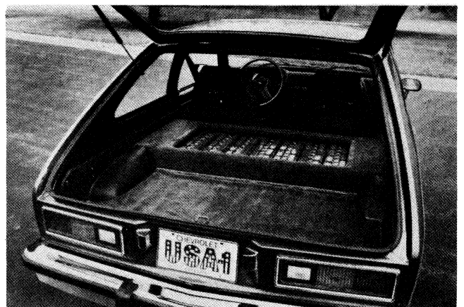
much as the conventional lead-acid battery pack at the right. On a pound-for-pound basis, the new cells can store more than twice the energy of the lead-acid cells. These batteries are shown installed in the rear of the Electrovette.
